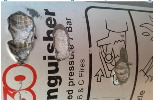
Figure 5 - Deep gouges in cylinder
