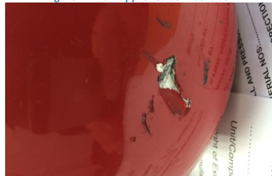
Figure 6 - Deep gouge in end cap
