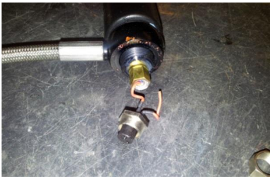
Figure 3 – Actuator damage due to “spanner checking”
