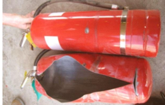
Figure 2 - Burst fire extinguisher due to dent and fatigue cracking (top extinguisher shows identical damage but has yet to reach failure point). These extinguishers are steel and were wall mounted on a ship (not a Lifeline cylinder)
